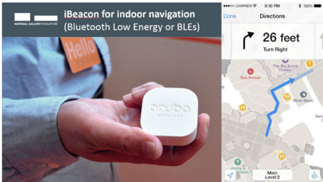
Fig 6. iBeacons offer potential of indoor navigation and trigger-based interaction. Image courtesy of Accenture.
